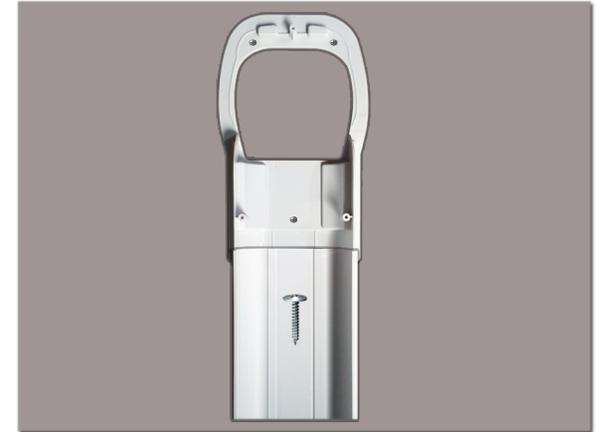
Align evenly and place the back tubing slightly inside the wall cover. Drill one hole (not predrilled) in the center of the tube and fasten with a screw. Secure backs of the coupler and/or elbow (if included) by fastening with the applicable screws into the middle predrilled holes.
